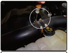
**4.** Losen the clamp on the intake system and pull back.
