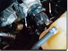
**22.** Install the 2.75" hump hose to the throttle body using provided clamps. Do not fully tighten yet.
