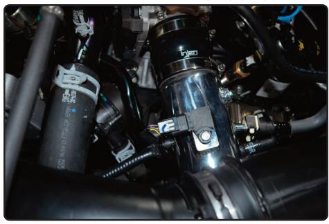
Congratulations! You have just completed the installation of this charge pipe. Periodically, check the alignment of the charge pipe, normal wear and tear can cause nuts and bolts to come loose. <u>Note: Check clearance and adjust if needed! Failure to check the alignment and adjust the charge pipe can cause damage that will void the warranty. Injen Technology is not responsible for any damages caused by/from improper installation.</u>
