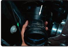
**12.** Pull back the plastic elbow from the intercooler.
