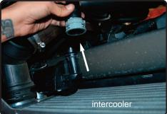
**10.** Twist and turn, the diverter valve hard line then pull back.
