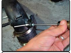
**19.** Remove the torx screw holding in the temperature sensor. Remove the sensor.
