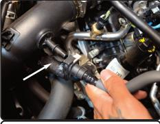
7. Disengage the crankcase line then pull back the line from the fitting on the charge pipe.
