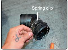
**15.** Remove the spring clip from plastic elbow.
