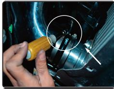
**24.** Attach the bottom part of the charge pipe and tighten using 8mm nut driver. Reconnect the diverter valve hardline. Reinstall coolant reservoir and reconnect intake system. Ensure all clamps and bolts are secured.
