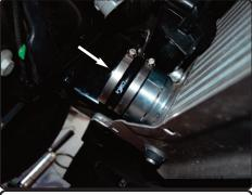
**18.** Attach the adaptor to the intercooler. Make sure you hear the click for the spring clips to be secured.
