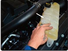
**3.** Carefully push aside the coolant reservoir.
