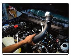
**13.** Remove the OEM charge pipe out of vehicle.
