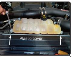
**2.** Remove the 2 bolts holding in the coolant reservoir.
