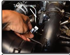
**8.** Disconnect the temperature sensor harness. Pull back the line from the charge pipe.
