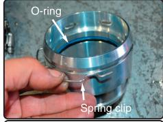
**16.** Install the o-ring and the spring clip to the billet adapter.
