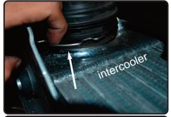
**11.** With a flat head screwdriver, pull back the spring clip, once removed. pull back the plastic elbow from the intercooler.
