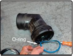
**14.** Using flat head screw driver remove the OEM o-ring from plastic elbow.
