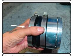
**17.** Install the 3.50" hump hose onto the adapter. Secure with the provided clamps.
