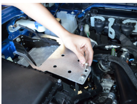
11. Secure the compressor bracket to the support bracket using the supplied nuts and bolts.
