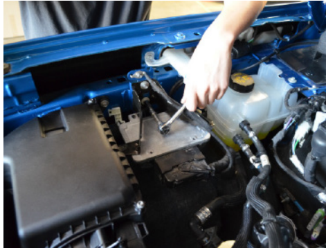
5. Remove the 2 bolts securing the OEM ECU bracket and the bolt securing the ground wire.
