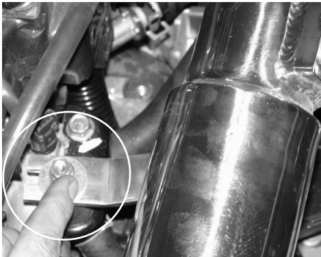
Use the fender washer and flange nut to secure the intake to the vibra-mount stud.
