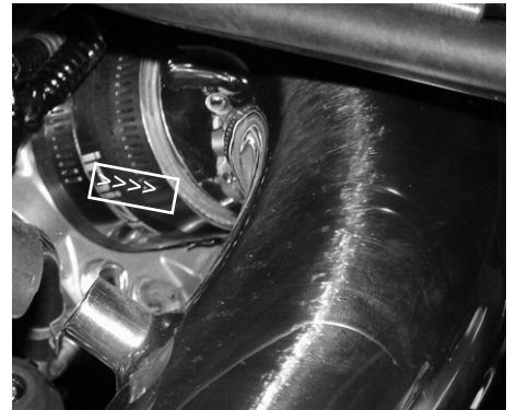
The top end of the intake is firmly pressed into the 2 1/2" hose while the clamp is semi-tightened.
