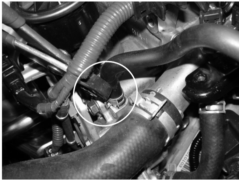
Using pliers, remove the tension clamp located on the upper coolant outlet hose running to the throttle body.
