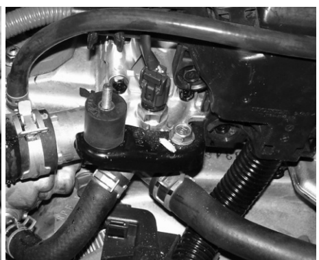
Screw the vibra-mount firmly into the brace until it sits flush on the brace.
