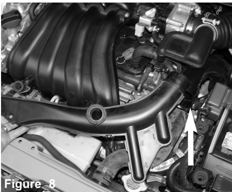
Figure 8 The resonator tube is now detached from the CCV box.
