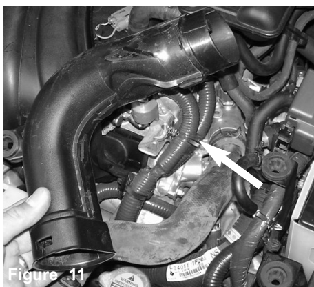
Figure 11 The air resonator tube is ready to be pulled from the engine compartment.
