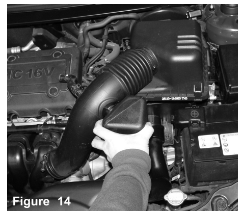
Figure 14 With all four retaining clips loose, remove the entire upper portion of the air box and air duct.
