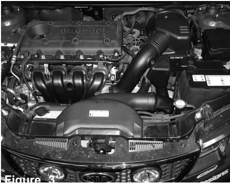
Figure 3 Stock air box cleaner and air ducts shown in this picture. Before getting started with the installation, be sure to disconnect the negative battery terminal.
