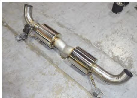
Figure 15 Re-install the hangers to the injen rear muffler assembly.
