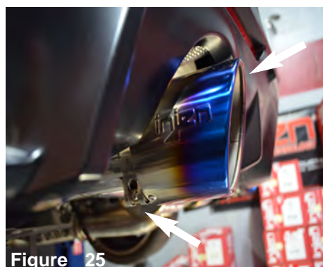
Figure 25 Now install the titanium tips to the rear muffler assembly. Secure and tighten and adjust to desired position.
