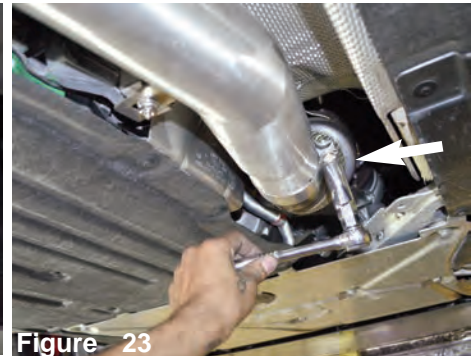
Figure 23 Once completed adjustment and clearance, tighten all clamps using 17mm and 13mm sockets. Readjust and reposition if necessary.
