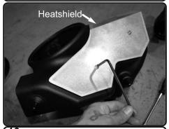
**19.** Install the heastshield to the bottom of the air box using provided M6 socket cap screws and tighten.
