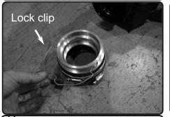
**11.** With the removed Lock clip, install into the new turbo on the outside like the OEM unit.
