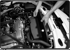
**10.** Install the heatshield into the vehicle. Position the grommet on heatshield to origi-nal air box fitting.
