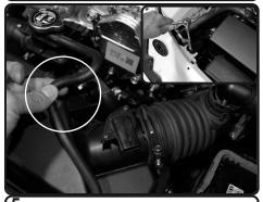
**5.** With 10mm socket and extension and ratchet, loosen the screw holding in the airbox on radiator support and clamp on throttle body. Pull back the coolant line from air box. Save screw for later install.
