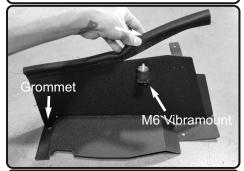
**9.** Install the Rubber trim to the top of heatshield. Install the M6 vibramount to the tab with thredded insert and secure. Install grommet to hole on heat shield.
