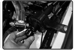
**23.** Install the provided vinyl cap to the sound tube muffler.
