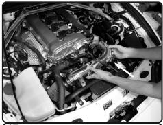
17. Install the 2.75" straight hose with clamps to throttle body. Now install intake tube assembly and position the tube to straight hose.
