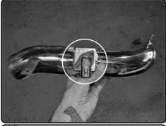
**15.** Secure using M4 button head screws and tighten using 2.5mm allen key.
