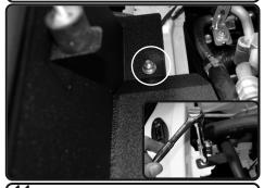
**11.** Secure the hole on heatshield to the M8 vibramount using provided M8 nut and washer. Secure the bracket using original screw from airbox and tighten.
