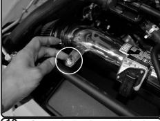
**18.** Secure the bracket on the intake tube to the vibramount on the heatshield using fender washer and M6 nut.
