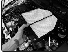
7. Now lift up and remove the bottom half of airbox.
