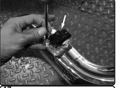
**17.** Now install the MAF sensor and secure secure using original screws.
