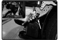
**8.** Loosen the bolts holding in thelower part of the air box resonator. Remove the upper rubber coupler out of vehicle.
