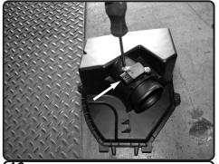
**16.** Loosen the 2 screws holding in the MAF sensor and remove.
