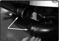
**9.** Loosen clamp on the lower part of the resonator connecting to scoop. Loosen and pull back.
