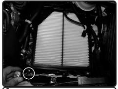
**6.** Now loosen the 2 bolts using 10mm socket or wrench and remove bottom half of airbox. Backside of airbox has grommet attached to fitting, pull hard for box to remove.
