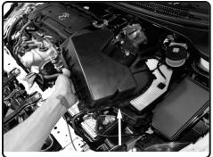
**5.** Loosen and remove the upper half of the air box.
