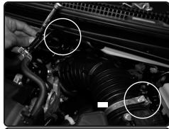
**3.** Using a 5.5mm socket, loosen both clamps on the airbox.
