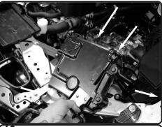
**13.** Do not disconnect ECU, pull back to sit on top of the radiator support.
