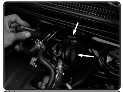
**14.** Now install the elbow hose with clamps to the throttle body, tighten clamp on throttle body only.
