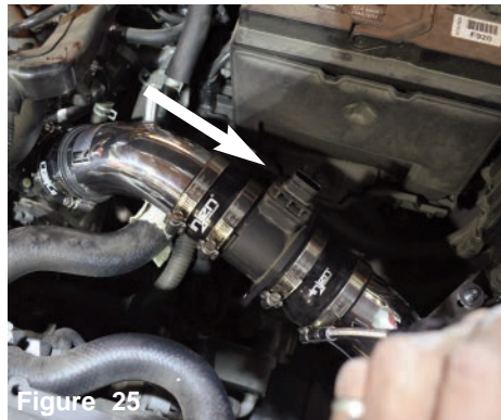
Figure 24 Using 8mm nut driver, tighten the clamp and secure.
