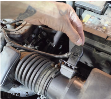
Figure 3 Disconnect the MAF sensor.
