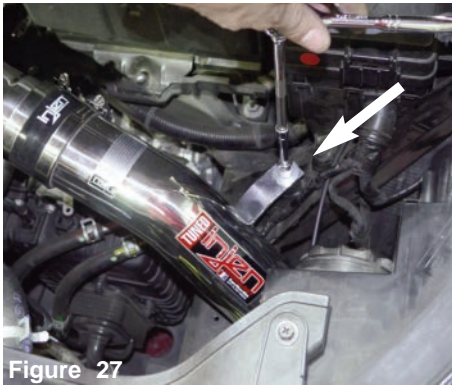
Figure 24 Using 8mm nut driver, tighten the clamp and secure.
