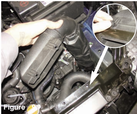
Figure 9 Remove the 2 push clips from the front of the radiator support holding in the ram scoop and remove.
