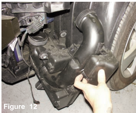
Figure 12 Pull any lines that are attached on or on the resonator and remove from the vehicle.
