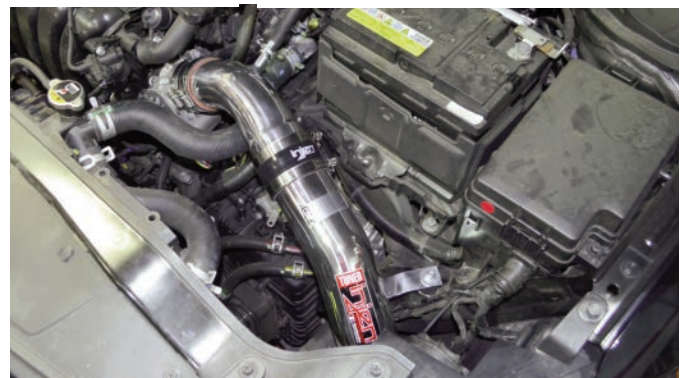
Figure 29 Secure using the factory clamp. Re-install bumper cover and connect battery terminals.
