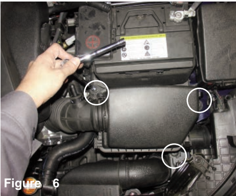
Figure 6 With 10mm socket and ratchet loosen the 3 screws holding in the air box assembly.
