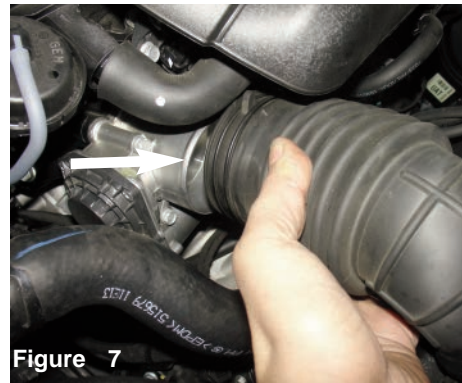
Figure 4 Now with pliers, loosen the clamp holding in crank case line and pull back.
