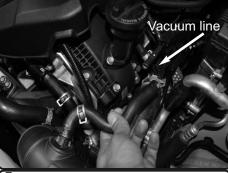
**5.** On driver side only, Loosen clamp and pull back vacuum line from engine.
