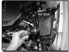
**3.** Loosen clamp on air box on both sides using 10mm socket or nut driver.
