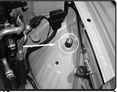
13. Install the provided vibramount to the original air box mounting insert on driver side. Secure and tighten.
