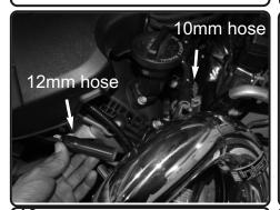
**16.** Install the provided 12mm hose to the crank case fitting and 10mm hose to the vacuum fitting.
