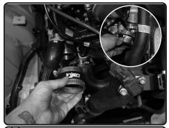
**14.** Install the provided 2-1/4" straight hose to the turbo on both sides with clamps. Tighten clamp on turbo only using 8mm nut driver.
