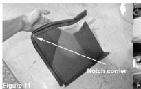
Now install the trim seal to the heat shield, For cleaner installation, notch corner with pliers or cutters.
