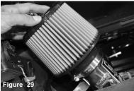
Now install the filter to the intake tube and tighten using 8mm nut driver. RE-install the factory scoop.
