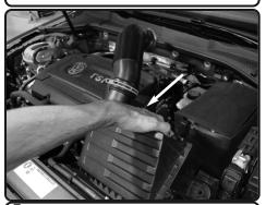
**5.** Now lift up OEM intake air box assembly out of vehicle.
