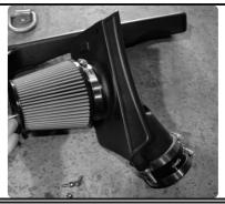
13 Install the filter to the plenum and tighten clamp with a 8mm nut driver.
