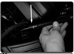
**23.** Connect the vacuum line and new hose together. This will have the extension to the brass 1/4" fitting on plenum.
