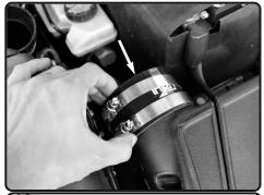
**18.** Install the 3.5" hump hose to the plenum. Do not Tighten.
