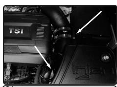
**24.** Now route the hose under the intake tube and connect to the 1/4" fitting.
