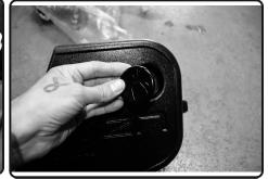
**11.** Install the filter minder plug into the filter minder hole cut-out on injen air box.
