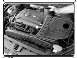
**16.** Install the intake assembly into the vehicle. Position to factory holes. Make sure the in-take assembly seats in studs. *Note:Use*
