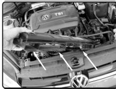
**8.** Now carefully pull back, and pull out the OEM ram-scoop from vehicle.
