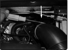
**3.** With 7mm nut driver, loosen the clamp on turbo housing.
