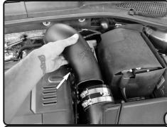
**19.** Install the intake tube to the vehicle. Position the tube to step hose and hump hose.
