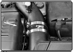
**21.** Tighten the hump hose using 8mm nut driver.
