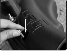
**14.** Install the plenum assembly into the air box. Secure using provided M6x20mm phillips screw with rubberized washer.
