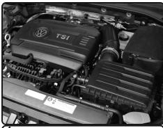
**1.** Stock box shown in this picture, if desired remove the engine cover for easier installation.
