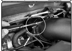
**20.** Position for the best fit. Tighten clamp using 8mm nut driver.
