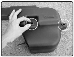
**12** Install the remaining 2 grommets to the holes on bottom of injen air box and secure.
