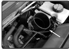
**10.** Install the 2-3/4"x3" step hose with clamps provided to the turbo housing.
