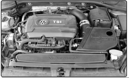
Congratulations! You have just completed the installation of this intake system. Periodically, check the alignment of the intake, normal wear and tear can cause nuts and bolts to come loose. <u>Note: Check clearance and adjust if needed! Failure to check the alignment and adjust the intake can cause damage that will void the warranty. Injen Technology is not responsible for any damages caused by/from improper installation.</u>
