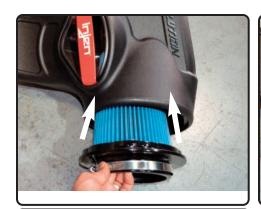
**12.** Install the new twist lock filter to the injen air box.
