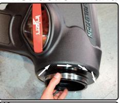
**13.** Once the filter is seated correctly, twist and turn in either direction a 1/4" turn.
