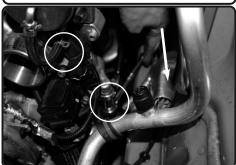
**30.** Tighten the 2 13mm bolts at the turbo using 13mm wrench.
