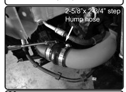
**20.** Install the 2-5/8" x 2-3/4" step hump hose with clamps to the intercooler and connect. adjust for clearance and fitment.
