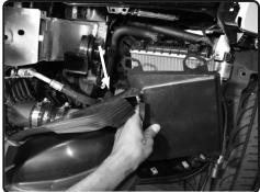
**22.** Secure and re-tighten the horn bracket and trans cooler. Re-install the trans cooler cover. Re-install bumper cover and re-connect sensors and camera.
