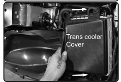
**8.** Slide the trans cooler cover over and remove.
