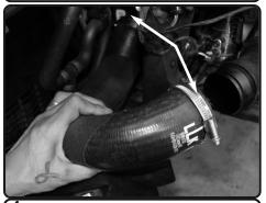
**4.** Once both sides are loosend, carefully remove the OEM hose out of vehicle.
