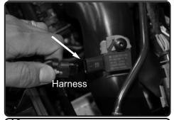
**10.** Disconnect the Temperature sensor harness.
