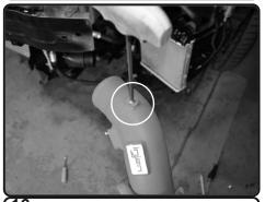
**16.** Install the provided 1/8" NPT plug to the fitting on the intake tube. secure and tighten using allen key. Install intercooler tube into the vehicle from bottom up and position.
