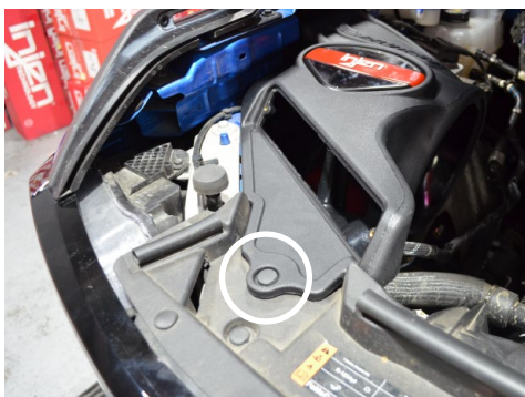
22. Secure the air box to the front shroud with the OEM push clip.
