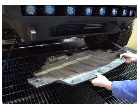
11. Remove the OEM skid plate.
