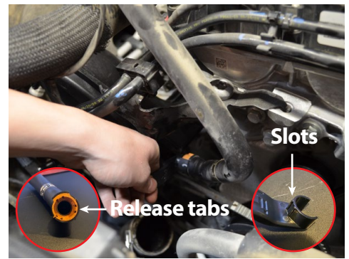
15. Line up the slots on the Injen release tool to the crank case fitting slots and then firmly pull the line. This will unlock the tabs required to release the fitting.
