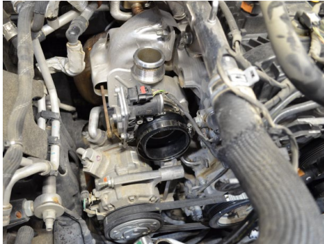
29. Attach the 2.50"-3.50" Stepping hump hose onto the turbo. Ensure the hose is properly seated before securing the clamp.
