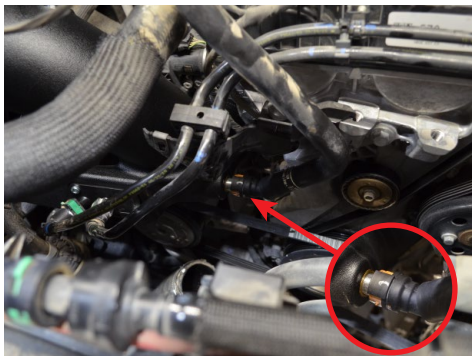
32. Reconnect the orange crank case line. A clicking sound will confirm it is properly secured.
