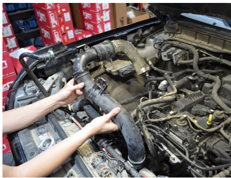
14. Remove the OEM intercooler pipe from the vehicle.
