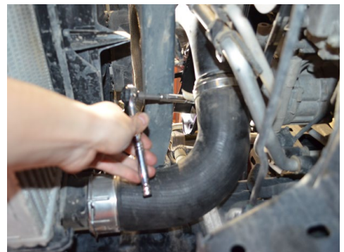
12. Loosen the clamp securing the bottom hose to the intercooler pipe.
