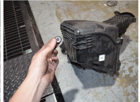
18. Remove the OEM grommet from the air box.
