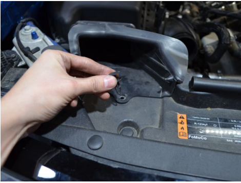
1. Remove the push clip securing the air box inlet to the front shroud.
