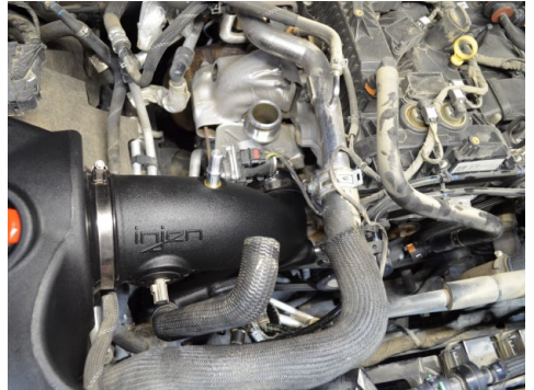
30. To install the injen intake tube, insert the tube into the hose then into the filter. Once in place secure the filter and hose clamp.
