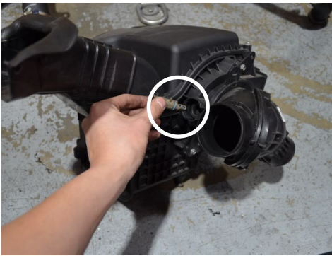
25. Lift the securing tab on the IAT sensor, then twist the sensor to remove it from the OEM air box.
