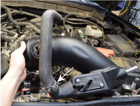
28. Install the OEM diverter valve hose onto the injen tube. Secure the hose with the OEM tension clamp.
