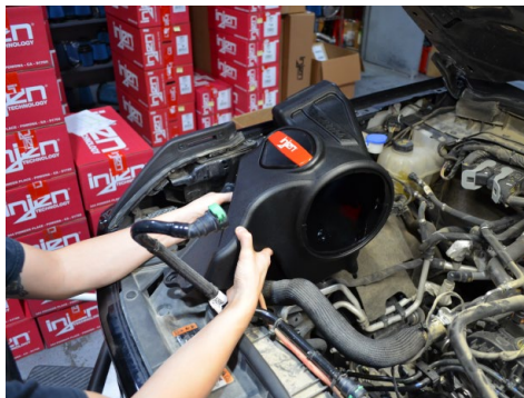
20. Line up the mounting pegs on the airbox to the grommets on the vehicle, then push down on the airbox.
