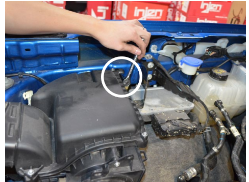
3. Remove the bolt securing the airbox to the chassis.
