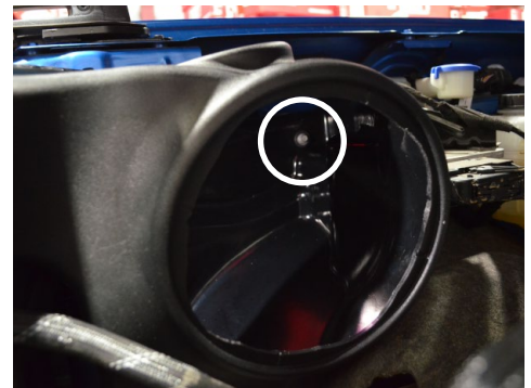
21. Reach into the airbox through the filter inlet to secure the air box to the chassis with the OEM bolt.
