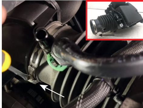
5. Loosen the clamp securing the intake hose to the intake tube.
