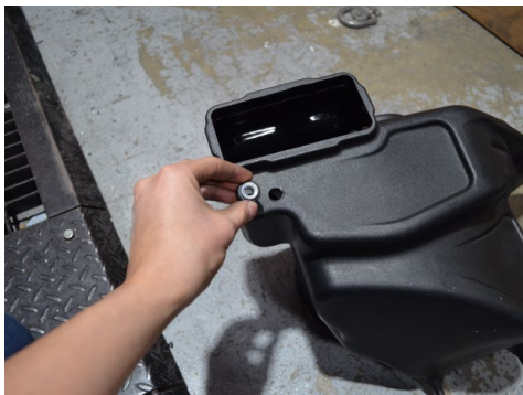
19. Install the OEM grommet on to the injen airbox.
