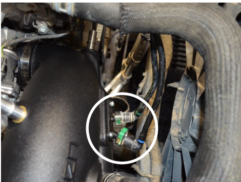
31. Reconnect the crank case lines to the intake tube ports. Reinstall the green locking clip.
