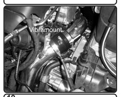
Connect the hose and adjust. Make sure the hoses are properly adjusted and clamps are behind the bead. This will prevent hoses popping off the pipe. Secure the bracket using provided washer
