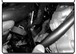
**32.** Secure the bracket using provided nut and fender washer. Secure and tighten using 10mm socket or wrench.
