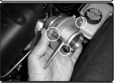
**9.** Loosen the 3 bolts holding in the OEM turbo adaptor using 5 mm allen key. Save the 3 bolts for later install
