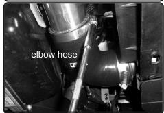
Adjust for fitment. Make sure all connections are properly secured. Re-route harness or lines. Readjust if necessary. Tighten all clamps using 8mm nut driver or ratchet. Tighten and secure the bracket using 10mm socket or wrench.
