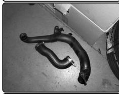
**7.** Complete hot side intercooler pipe out of vehicle.
