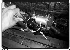
**21.** Loosen the clamp on throttle body using 7mm nut driver or ratchet.
