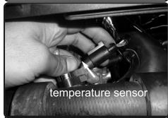
**31.** Re-connect the temperature sensor harness.
