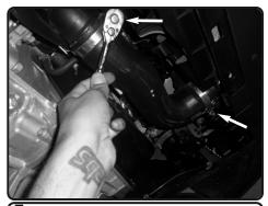
7. Loosen 2 clamps on the lower part of the hot side of the intercooler hose using 7mm socket or nut driver.
