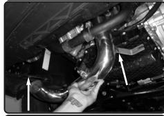
**30.** Install the cold side intercooler pipe into the vehicle. Positon to the throttle body and bracket to the vibramount.
