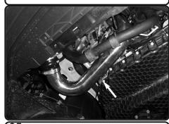
**35.** Secure and tighten clamps using 8mm nut driver. Re-install guard, and intake system. Your intercooler pipe kit is now complete.
