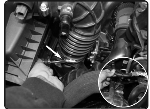
4. Loosen the clamp on the turbo plastic inlet. Pull back the line attached to the intake tube.
