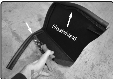
9. Install the trim seal. Notch corner for easier installation with pliers.
