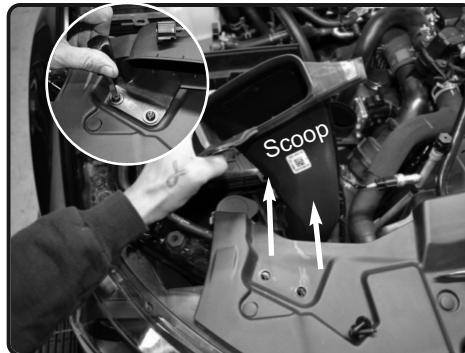
7. Loosen the 2 bolts holding in the OEM scoop. lift up and remove the scoop.
