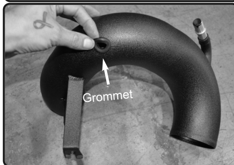
11. Install the grommet to the hole on the intake tube.
