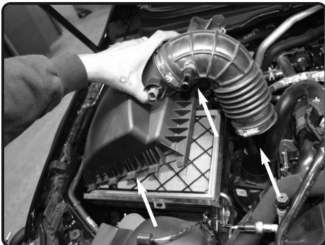
5. Lift up and remove the upper half of the air box assembly.
