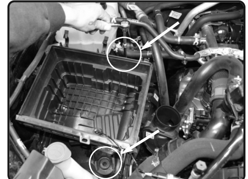
8. Loosen and remove the 2 bolts holding in the lower part of the air box using 8mm socket or wrench. Remove the lower air box out of the vehicle.
