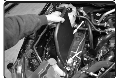
12. Install the heatshield into the vehicle and position the tabs to the threaded inserts from step 8.
