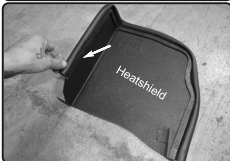
10. Make sure trim is on and secured properly.
