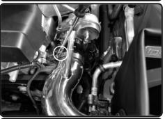
**23.** Now once positioned for best fit, tighten the clamp on step hose and secure using 8mm nut driver.
