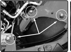
**12.** Secure all 3 vibramounts and tighten using 10mm wrench.
