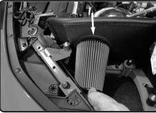
**20.** Install the filter and position to in-take tube.
