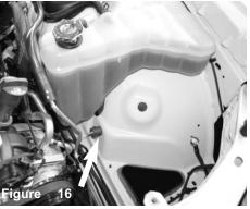
Place a vibramount on the pre-drilled hole on the inner wheel well in the engine bay. You will have to secure the vibra mount from the outer wheel well using a supplied M6 nut. Figure 17 will illustrate how
