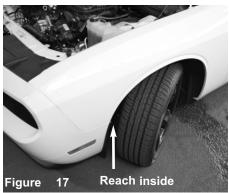
Turn the steering wheel to the left. This will give you access to the outer wheel well to secure the M6 nut to the vibramount from figure 16. No wrench neccessary, just turn the vibramount until it's snug.
