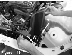
(A) Align the front heatshield tab to the bracket on the front radiator support. A vibramount will be used to secure them together in the next step. (B) Align the hole in the back of the heatshield to the vibramount from figure 16.
