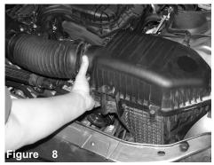
Now lift up and remove the complete stock air box assembly
