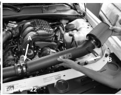
(A) Position the other end of the secondary tube into the primary tube from figure 15 (B) Also, Align the Bracket on the secondary tube to the vibramount on the radiator support from figure 20.
