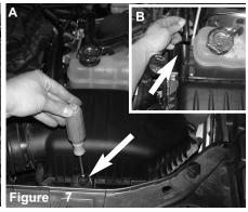
Figure A: Pull back the crank case line from the stock air box. <u>Figure B:</u> Disconnect the crank case breather line from the air box assembly
