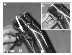
Figure A: Place the sensor grommet into the drilled hole located at the end of the intake pipe. Figure B: Grommet installed in hole
