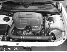
Align the entire intake for the best possible fit. Once you have rechecked and cleared the intake from all moving parts, continue to tighten all nuts, bolts and clamps.
