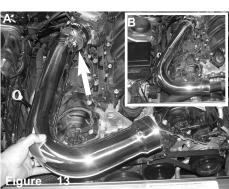
Figure A: Place the primary pipeinto the 3 1/8" hose located on the throttle body. Figure B: Pipe shown in proper position
