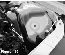
(A) Once the heatshield is aligned, place a vibramount onto the front heatshield bracket to secure it to the bracket on the front radiator support. (B) Use a M6 nut to secure the back of heatshield to the vibramount from figure 16.
