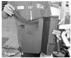
Place the 8" vinyl trim onto the right side of the heatshield and the 18" vinyl trim onto the top side.
