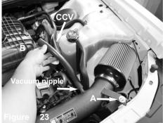
(A) Use a M6 nut and fender washer to secure the intake bracket to the vibramount. Make your final adjustment and secure the clamp on the hose in figure 5 (B) Use the 10"-15mm vacuum hose and connect the vacuum nipple on the intake tube to the crank case vent tube
