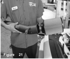
Place the filter onto the bracket end of the secondary tube
