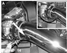
Figure A: Place the air temp sensor into the sensor grommet located near the throttle body. Figure B: Sensor plugged into grommet
