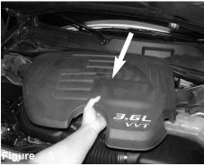
Lift up and detach the engine cover from the engine
