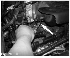
Rotate and twist the air temp sensor off of the air duct Remove the air duct from the throttle body. located on the left side of the throttle body.
