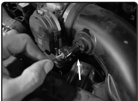
5. Disconnect the temperature sensor harness
