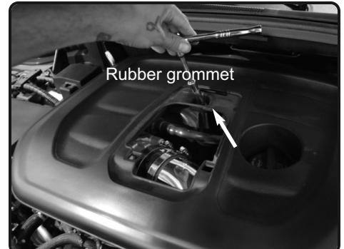
**28.** Install the engine cover and secure.
