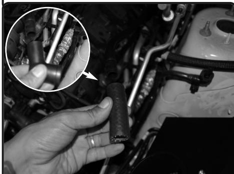
**20.** Remove the rubber elbow coupler from the crankcase plastic line. Install provided 15mm hose.
