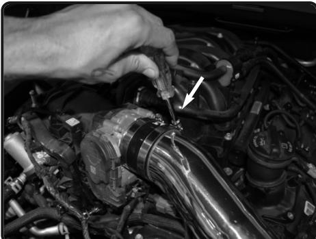
**25.** Secure and tighten clamp on throttle body.
