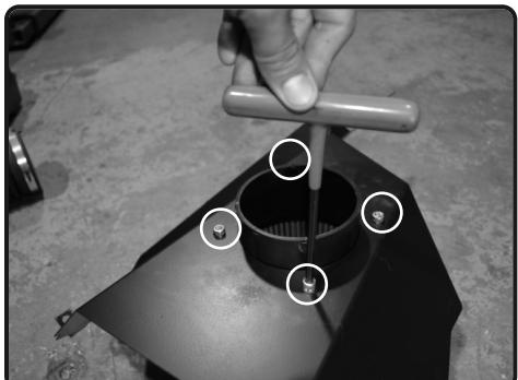
**13.** Install the provided adaptor to the inside of the heatshield. Secure using provided M6 socket cap screws.
