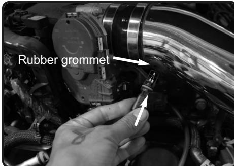
**26.** Install the temperature sensor to the grommet on intake tube and secure. Re-connect the harness.
