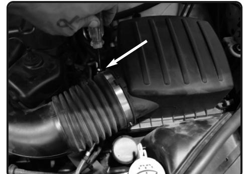
4. On the air box, loosen the clamp.
