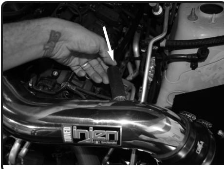
**27.** Connect the crank case line to the fitting on intake tube.
