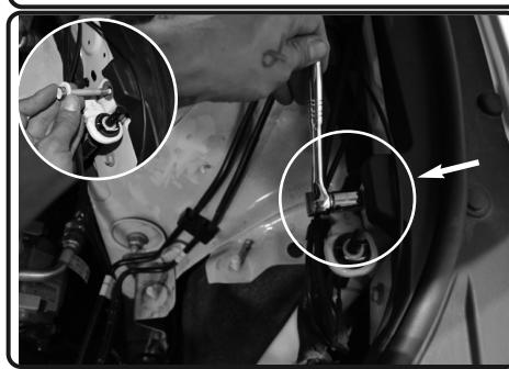
11. Loosen the bolt on the side of the fender compartment next to the hood push pin. Remove bolt and save for later install.
