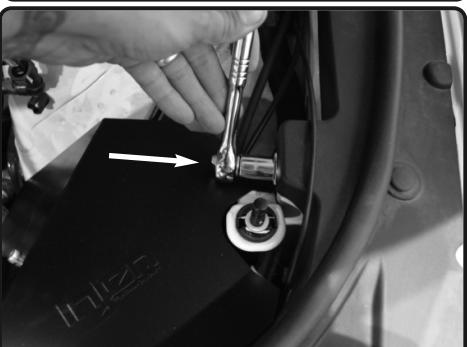
**18.** Re-install the bolt from step 11 and secure the heatshield.
