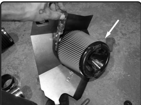
**14.** Install the air filter to the adaptor and secure using 8mm nut driver.
