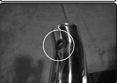
**22.** Install the provided rubber grommet to the hole on the intake tube.
