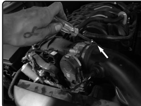
3. Loosen the clamp on the throttle body.
