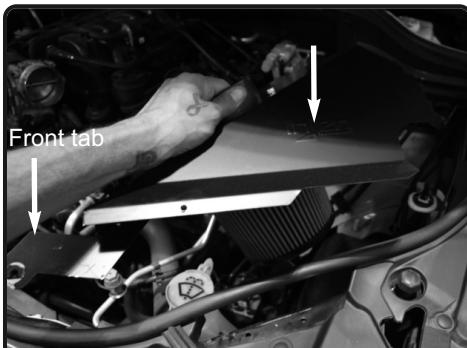
**16.** Install the heatshield assembly into vehicle and position. Make sure the front tab goes under the plastic shroud.
