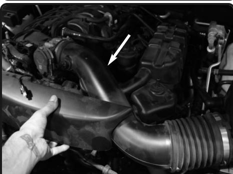
6. Remove the intake tube out of vehicle.
