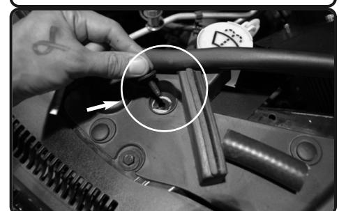
12. Loosen the 10mm bolt on the radiator support.
