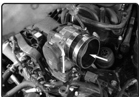
**21.** Install the provided straight hose with clamps to the throttle body.
