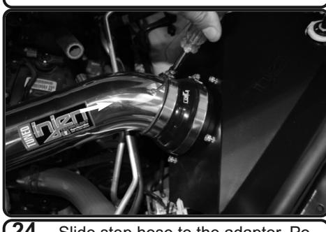
**24.** Slide step hose to the adaptor, Position for best fit. Secure and tighten.
