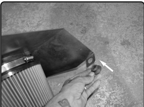
**15.** Install the grommet from step 9 to the lower tab with hole cut out on heatshield.
