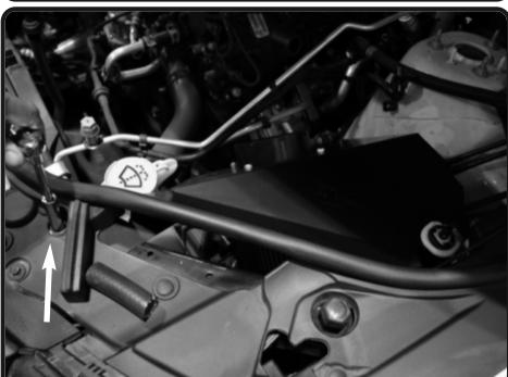
**19.** Re-install the bolt from step 12 and secure the heatshield tab under the plastic shroud cover.
