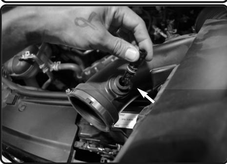
10. Turn and remove the temperature sensor out of the intake tube.
