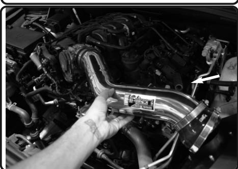
**23.** Install the step hose to the intake tube with clamps and slide back. Install the intake tube to the vehicle and position to straight hose and adaptor
