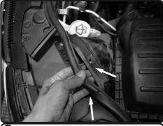
7. Carefully pull back the rubber hood line trim from the air box ram inlet.
