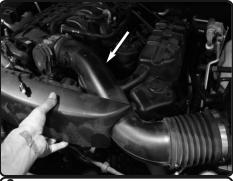
**6.** Remove the intake tube out of vehicle.
