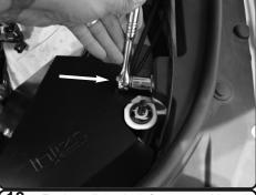
**18.** Re-install the bolt from step 11 and secure the heatshield.
