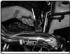
**27.** Connect the crank case line to the fitting on intake tube.
