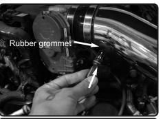
**26.** Install the temperature sensor to the grommet on intake tube and secure. Re-connect the harness.
