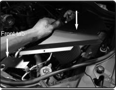
**16.** Install the heatshield assembly into vehicle and position. Make sure the front tab goes under the plastic shroud.
