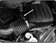
**4.** On the air box, loosen the clamp.
