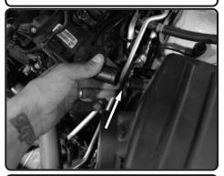
**8.** Pull back the crank case line from the air box.
