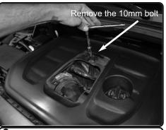
**2.** Loosen the cover cap and loosen the bolt holding in the engine cover. Lift up and remove the engine cover.
