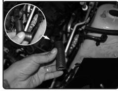
**20.** Remove the rubber elbow coupler from the crankcase plastic line. Install provided 15mm hose.
