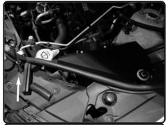
**19.** Re-install the bolt from step 12 ansd secure the heatshield tab under the plastic shroud cover.
