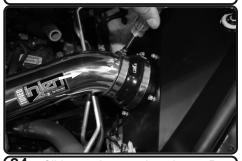
**24.** Slide step hose to the adaptor, Position for best fit. Secure and tighten.
