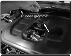
**28.** Install the engine cover and secure.
