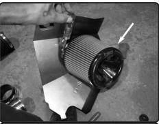
**14.** Install the air filter to the adaptor and secure using 8mm nut driver.
