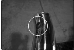
**22.** Install the provided rubber grommet to the hole on the intake tube.
