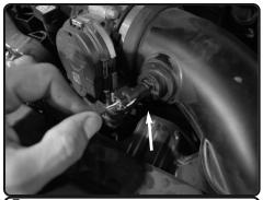
**5.** Disconnect the temperature sensor harness
