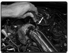
**25.** Secure and tighten clamp on throttle body.
