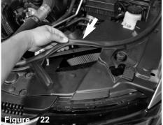
Attach the green tree push pin on the trim seal into the hole on the heatshield scoop inlet.
