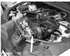
Lift up and remove the air box assembly from the vehicle
