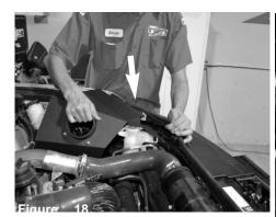
Lift up the plastic radiator support cover and slide the heatshield bracket under it to its mounting position. The mounting position will be the bolt from figure 14. The heatshield will be secured later.
