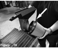
Place the filter onto the velocity stack and then secure the clamp.
