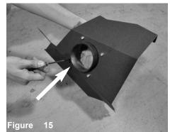
Secure the velocity stack to the heatshield with four M6 socket cap screws.
