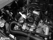
Now tighten the clamp on the throttle body using 8mm nut driver. Secure and tighten.
