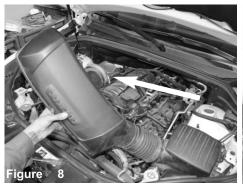
Now lift up and remove the complete stock intake tube.
