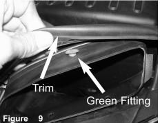
Carefully pull out the weather trim from the scoop, green fitting that can move from left to right.
