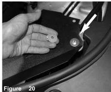
Secure the heatsheild using provided M6 screw fender washers and M6 lock nut.
