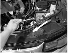
Temporarily remove this 10mm bolt from the radiator support. This bolt will secure the Injen heatshield to the radiator support later in <u>figure 12</u>.
