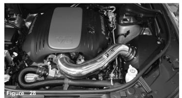
Congratulations! You have just completed the installation of this intake system. Periodically, check the alignment of the intake, normal wear and tear can cause nuts and bolts to come loose. <u>Note: Check clearance and adjust if needed! Failure to</u> check the alignment and adjust the intake can cause damage that will void the warranty. Injen Technology is not responsible for any damages caused by/from improper installation.
