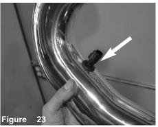
Remove the temperature sensor out of the OEM airbox. Install grommet to the intake tube hole. Now install and secure the Temperature sensor to the grommet.
