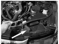
Line up the hole on the bracket of the heatshield to the location where the bolt was removed from figure 6. Reuse the O.E. 10mm bolt to secure the heatshield bracket to the radiator support.
