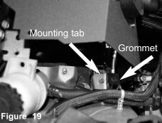
Place the grommet on the heatshield onto the O.E. air box mounting tab on the chassis. Use the power steering reservoir in the photo for reference to locate the mounting tab in the photo.
