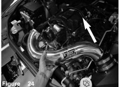
Install the intake tube into the vehicle. Position the tube Position for the best fit, tighten all the clamps. to the adaptor and the hose on throttle body.
