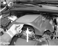
Lift up and remove the engine cover.
