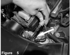
Disconnect the Temperature sensor and remove the sensor from the intake tube.
