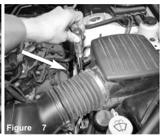
Loosen the clamp on the air box.
