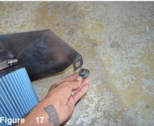
Remove the OEM grommet from the OEM air box and place the grommet onto the mounting tab.
