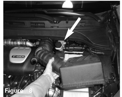
Figure 8 Remove the entire upper air box assembly and air duct from the engine bay
