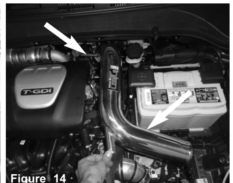
Figure 14 Position the intake pipe into the engine bay and place the end of the pipe into the step hose on the turbo compressor outlet.
