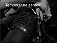
**3.** Disconnect the temperature sensor harness.
