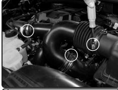
**4.** Loosen the 3 clamps on the stock intake tube using 7mm nut driver.
