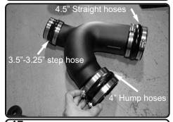
**17.** Place the supplied hoses illustrated in the photo. The # 72 clamp will be used on the 4.0" hump hose and 4.5" straight hose and #64 and #56 clamps will be used for the 3.5"- 3.25" step hose.
