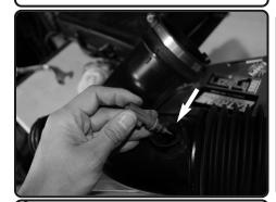
**9.** Loosen and remove the temperature sensor out of stock intake. Use a small flat head screwdriver to pull back clip on sensor.
