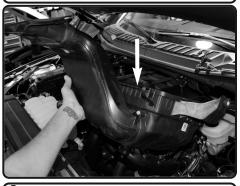
**8.** Now lift up and remove the bottom half of air box out of vehicle.
