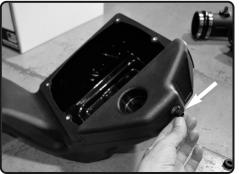
**10.** Remove the grommet and spacer from the OE lower air box and re-install it in the Injen lower air box.
