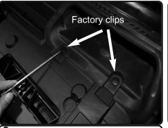
**2.** Remove the two plastic retaining rivets from the air scoop and remove scoop from engine bay.
