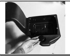
**11.** Install the Filter Minder plug into the lower air box assembly
