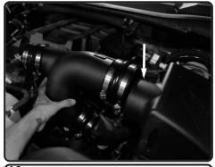
19. Install the Injen intake tube to the factory intake tubes and then connect the Injen in-take tube the the Injen intake air box. Make your final adjustment and then secure all the clamps
