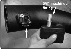
11. Install the MAF sensor into the tube. Secure and tighten the MAF sensor using provided M4 button head screws. MAke sure fitting is installed and secured.
