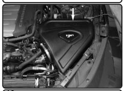
**12.** Now install the air box into the vehicle. Position the tabs on air box to OEM grommet locations.
