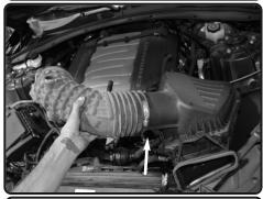
**7.** Now lift up and remove the OEM intake system out of the vehicle.
