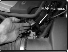
**2.** Disconnect the MAF sensor harness and pull line away from the intake tube.
