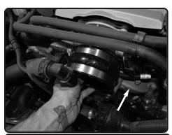
**13.** Install the 4" hump hose with clamps to the throttle body. Tighten clamp on throttle body only.
