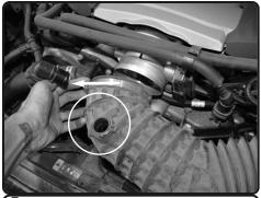
**5.** With pliers or flathead screwdriver, pull back the clamp to the sound tube fitting and pull back from the intake tube a
