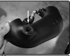
14. Install the large grommet to the hole on the intake tube
