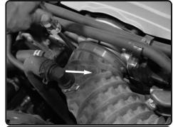
**3.** With 8mm nut driver, loosen the clamp on the throttle body and pull back tube.
