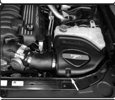
**18.** Secure and tighten the air box screw from step 10
