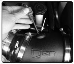
**16.** Install the temperature sensor to the grommet on intake tube and secure.
