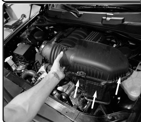
6. Carefully lift up and remove the stock air box assembly.
