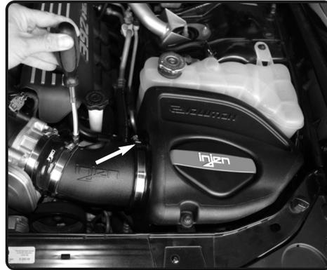
**14.** Adjust for fitment and tighten all clamps using 8mm nut driver.
