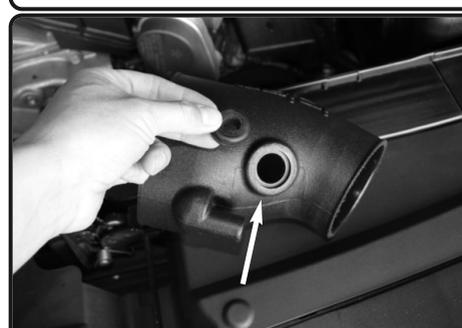
11. Install the provided grommet to the hole on the intake tube.
