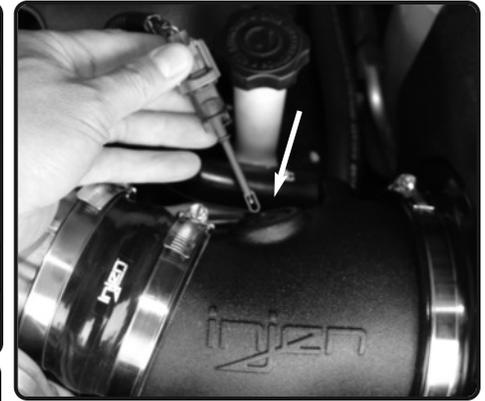
**16.** Install the temperature sensor to the grommet on intake tube and secure.
