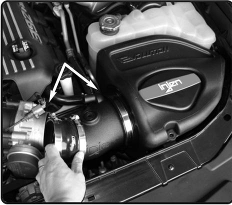
**13.** Install the intake tube to the filter and the hose to the throttle body.
