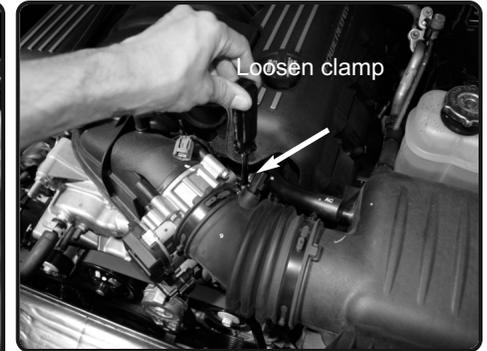
4. Loosen the clamp on throttle body using 8mm nut driver.
