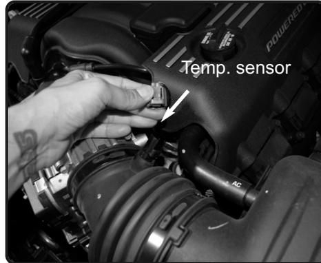
2. Disconnect the Temperature sensor harness.
