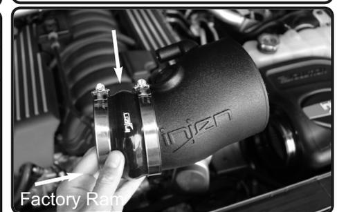
12. Install the provided 3.5" hump hose with clamps to the intake tube.
