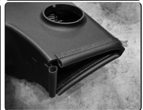
8. Install the provided bulb trim to the bottom of the airbox.
