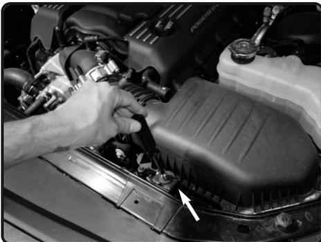
5. Loosen the bolt holding in the airbox using 8mm nut driver.
