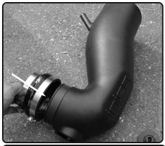
**13.** With provided Step hose and clamps install to the tube. Do not tighten.
