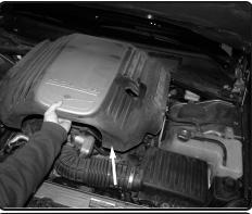
**2** . Lift up and remove engine cover.
