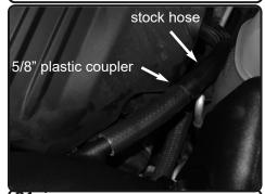
**21.** Install the provided 17mm hose and plastic coupler to the stock crank case hose. Connect the two and secure to the intake tube
