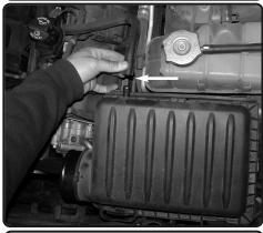
**7.** Pull back the crankcase line from the airbox fitting.
