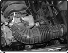
**5.** Loosen the clamps on the air box and throttle body using 8mm nut driver.
