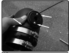
**15.** Secure the temp adaptor using the provided m4 button head screws. Tighten using 2.5mm allen key.
