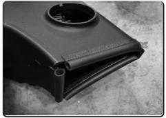
**10.** Install the provided bulb trims to the bottom of the airbox.
