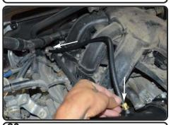
**23.** Remove the smaller vacuum line, install the provided 4mm vacuum line and secure to engine and fitting on intake tube. Re-install the engine cover.
