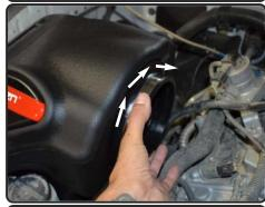
**19.** Once seated, rotate in either direction 1/4 turn till filter locks.
