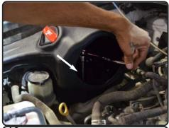
**16.** Secure the OEM airbox to the original airbox position.
