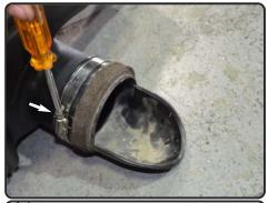
**14.** Secure using provided #56 band clamp.
