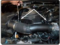
7. With 10mm nut driver or socket with ratchet, loosen the clamps on throttle body and airbox.
