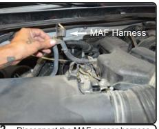
**2.** Disconnect the MAF sensor harness and pull line away harness from the airbox.
