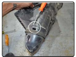
**12.** Carefuly remove the OEM Air box scoop using flathead screwdriver.
