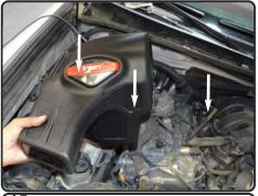
**15.** Install the air box assembly into the vehicle and position.
