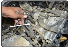
**10.** Loosen and remove the harness bracket from the engine using 10mm socket or wrench.
