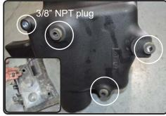
**11.** Remove the 3 grommet with crushwasher and install into the new air box. Install the provided 3/8" NPT plug to the thredded hole on the air box.
