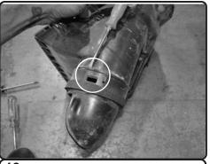
**13.** Carefully remove the OEM Air box inlet scoop using a flathead screwdriver.
