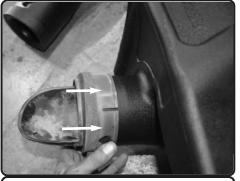
**14.** Install the OEM inlet scoop onto the Injen air box inlet.
