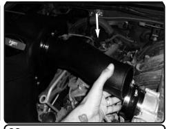
**22.** Install step hump hose to the throttle body. Install the intake tube to the vehicle and position.
