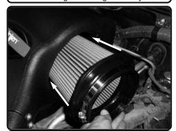
**20.** Insert twist lock filter to the air box.
