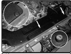
**19.** Position the scoop and make sure the smaller holes are used for the 2 push clips from step 10. The 2 hood bushings will go through the scoop.
