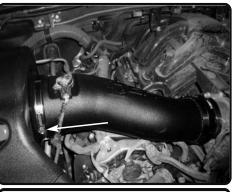
**25.** Tighten all clamps using 8mm ut driver. Re-install the engine cover.
