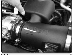
**14.** Slide the hose onto the throttle body and position the intake tube and airbox into place.
