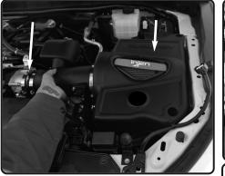
**13.** Attach the provided 3-1/2" hump hose with clamps to the intake tube and install the intake assembly.
