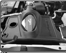
**15.** Secure the airbox using OEM screws and tighten. Adjust intake tube and tighten clamps using 8mm nut driver.
