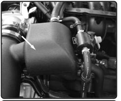
**16.** Re-connect the Crank case lines to the injen catch can. Secure using OEM clamps.
