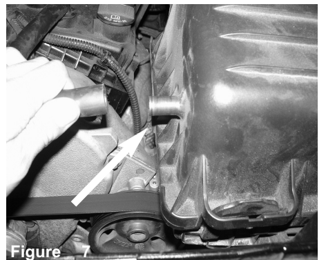
Figure 7 Pull back the crank case line from the stock air box.
