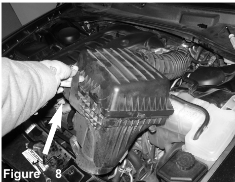
Figure 8 Now lift up and remove the complete stock intake system.
