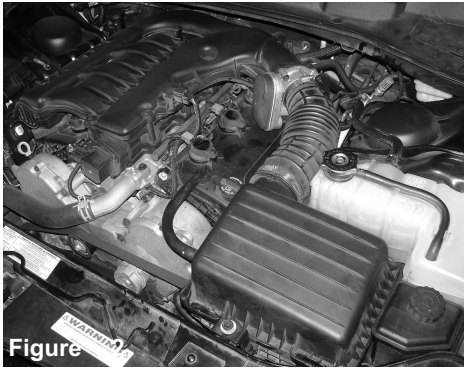
Figure 1 Complete stock air intake cleaner and air intake duct.
