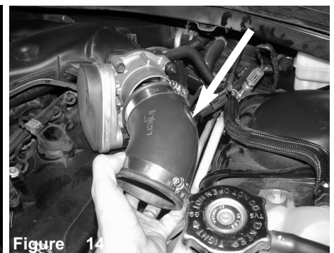
Figure 14 Install the elbow with clamps provided to the throttle body. Make sure the 2-3/4 inch side is installed on the throttle body.
