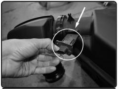
**4.** Remove the 2 screws holding in the MAF sensor using T25 torx bit.
