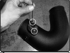
**5.** Install the MAF sensor in the correct direction. Secure using the provided M4 screws. Tighten using 2.5mm allen key.
