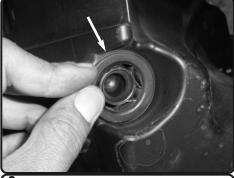
**6.** Remove the factory grommet fitting plug from the bottom of the airbox.
