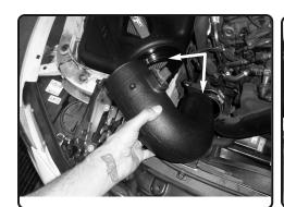
**12.** Install the intake tube and position to the filter and the tube to the turbo.
