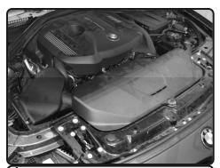
**1.** Stock intake system shown. Lift up and remove engine and the front radiator cover.
