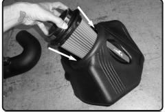
**9.** Install the twist lock filter into the injen air box.
