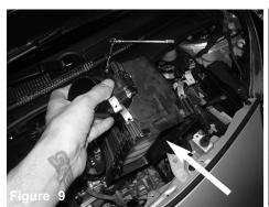
Now lift up and remove the air box and filter out of the vehicle.
