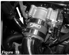
Position for the best fit, secure the bracket using provid- Position for best fit and tighten using 8mm nut driver.
