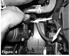
Disconnect the MAF sensor harness, pull harness away from the air box.
