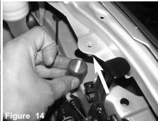
Now install the vibra mount from the bottom up towards the thredded insert located on the radiator support.
