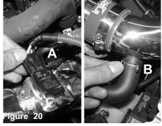
A) Re-connect the MAF sensor harness. B) Attach the crank case line to the fitting on the intake tube.
