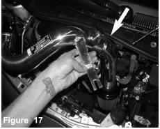
Install the intake assembly into the vehicle and position the bracket to the vibra mount and to the throttle body.
