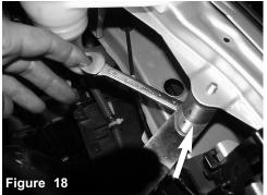
Position for the best fit, secure the bracket using provided M6 nut and fender washer. Tighten using 10mm wrench
