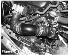
With 10mm socket and wrench, loosen the clamps on the throttle body and the air box.
