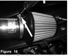
Install the air filter to the intake tube and tighten using 8mm nut driver.
