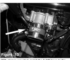
With clamps provided, install the 2-3/8" hose to the throttle body and position. Tighten the clamp on the throttle body only using 8mm nut driver.
