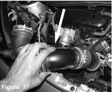
Now remove the stock intake tube from the vehicle.
