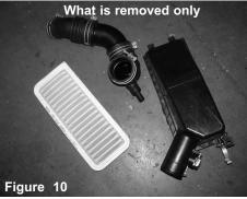
The bottom half of the OEM air box is molded to the radiator shroud. That will stay in place and not be removed.
