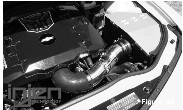
Your intake system completely installed. Check all fittings and connections. re-tighten clamps if necessary. Thank you for choosing injen.
