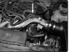
11. Install thje intake tube assembly and position the tube to throttle body and hump hose on plenum.
