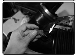
**8.** Loosen and remove the temperature sensor out of stock intake. Use a small flat head screwdriver to pull back clip on sensor.
