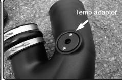
11. Install the temperature sensor adaptor to the intake tube and secure using provided M4 button head screws. SEcure and tighten using 2.5mm allen key.
