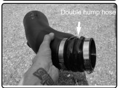
**9.** Install the provided double step hump hose to the intake tube with clamps provided.
