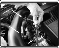
19. For the 3.5.L and Raptor models, pull back the Temp harness clips from the intake tube, this will allow for more length to the sensor. Re-connect Temp harness.
