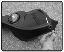
**12.** REmove the OEM grommet and crush washer from the stock airbox. Install into the new injen air box.
