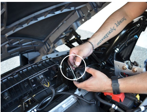
10. Replace the OEM bolt holding the car horn with the provided M6X20mm bolt.
