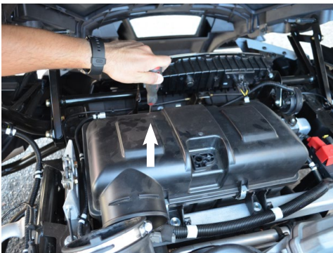
7. Remove the bolt holding down the front of the OEM air box.
