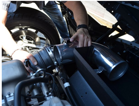
17. Insert the injen tube into the OEM hose. Leave the OEM clamp loose for now.
