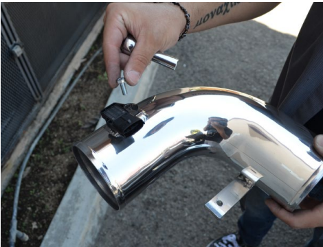
16. Install the IAT sensor onto the injen tube, then secure using the provided M6X15MM hex bolt.
