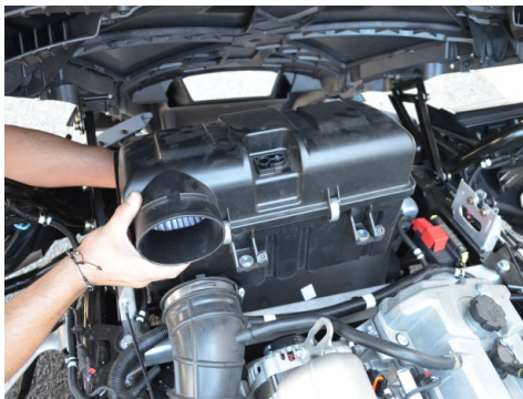
8. Remove the stock air box from the engine bay.
