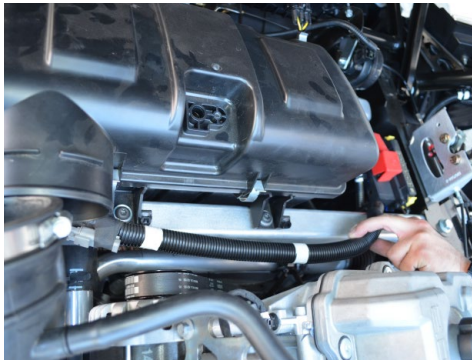
5. Detach the harness from the air box.
