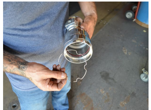
21. Install the retaining clip onto the cold side intercooler pipe.
