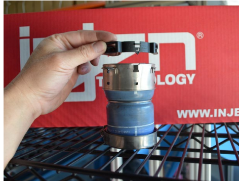
5. Remove the plastic retaining clip from the hot side turbo outlet coupler by carefully prying on both ends and then lifting up.
