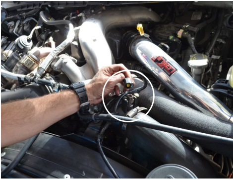
13. Disconnect the IAT sensor harness located on the OEM cold side intercooler pipe.
