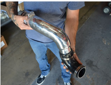
22. Install the elbow hose onto the cold side intercooler pipe. Secure using the provided clamps.
