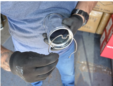
7. Install the OEM retaining clip onto the Injen secondary hot side intercooler pipe.
