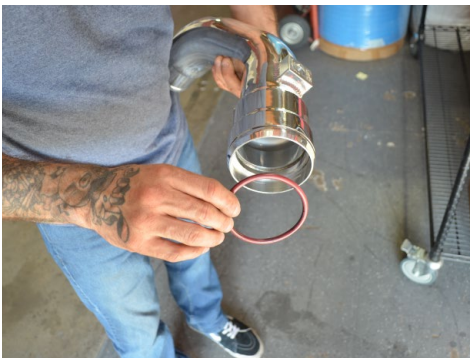
19. Install the OEM O-Ring onto the Injen cold side intercooler pipe in the same direction it was removed.
