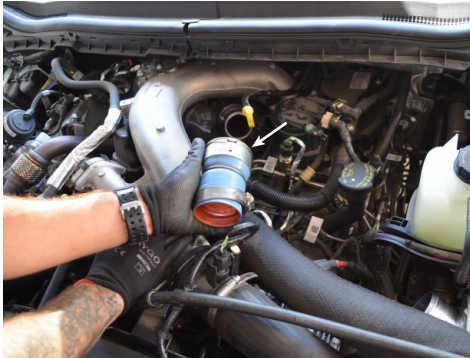
4. Disengage the retaining clip attached to the turbo outlet by prying up on the retaining clip then remove the hot side turbo outlet coupler.
