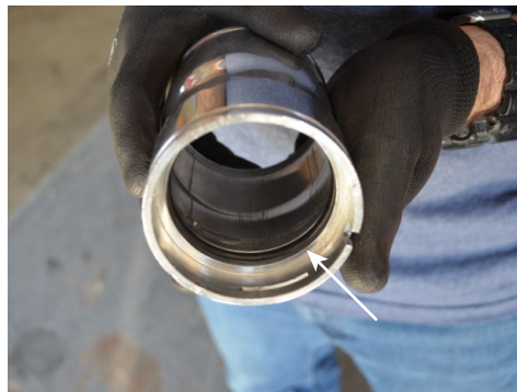
8. Install the provided O-Ring onto the secondary hot side intercooler pipe.
