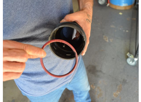
18. Remove the O-Ring from the IAT sensor adapter. Note the direction it was removed in.
