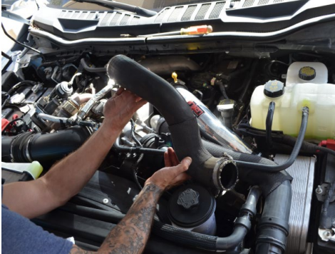
16. Remove the cold side intercooler pipe from the engine bay.
