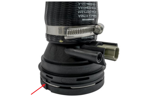
20. Remove the OEM retaining clip from the IAT sensor adapter.
