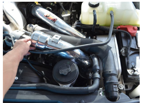
24. Once the intercooler pipe is in place. Secure the clamp then secure the power steering reservoir to its factory location.
