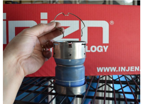
6. Remove the retaining clip from the hot side turbo outlet coupler.
