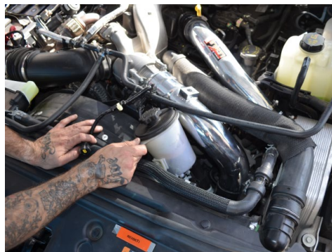
23. Remove the bolt securing the power steering reservoir then move the reservoir to give clearance for installing the intercooler pipe.
