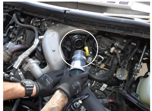
9. Install the secondary hot side intercooler pipe onto the turbo outlet. You should hear the retaining clip engage.
