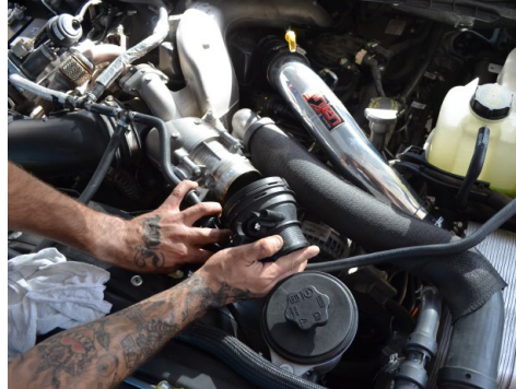
17. Disengage the retaining clip from the IAT sensor adapter then remove the adapter from the engine bay.
