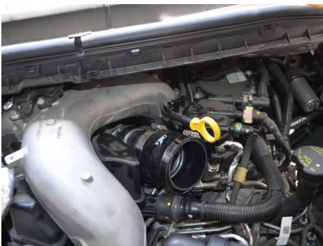
10. Install the 3.00" hump hose onto the secondary hot side intercooler pipe. Secure using the provided clamps.
