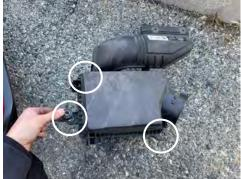
**10.** Remove the three grommets and spacers from the stock air box assembly. Grommets will be used on the Injen air box
