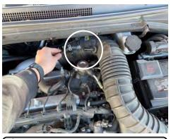
**4.** Disconnect the vacuum line on the stock intake tube
