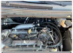
**15.** Place the 2.75"-3.50" step hose, #44 and #56 clamp onto the turbo inlet. Secure only the 2.75" hose end to the turbo inlet using the #44 clamp for now
