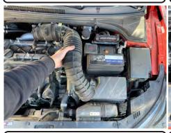
**5.** Loosen the clamps at each end of the intake tube and remove the tube
