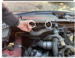
**9.** Remove the two screws from the front scoop bracket and then remove the scoop bracket
