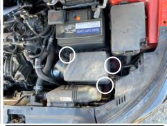
**7.** Remove the three 10mm bolts from the factory air box assembly
