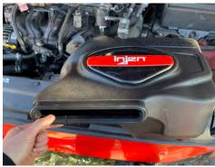
**12.** Install the 18" vinyl trim onto the Injen air box inlet
