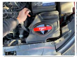
**13.** Lower the air box into the engine bay and secure it using the three original 10mm bolts
