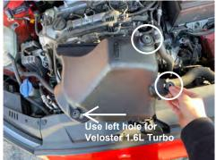
11. Place the three grommets from figure 10 onto the Injen air box. Note: Confirm grommet location on the Veloster models in the photo
