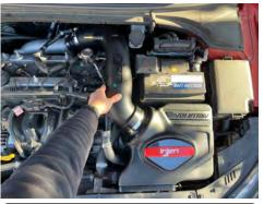
**16.** Place the Injen intake tube into the 2.50" hose end and the other end of the tube into the filter inlet
