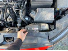
**6.** Press the two pins on the plastic rivets on top of the factory inlet scoop and then remove the rivets
