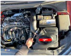
**19.** Tighten all hose clamps on the intake assembly
