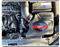
**17.** Reattach the diverter valve return line to the Injen Intake tube diverter valve port.
