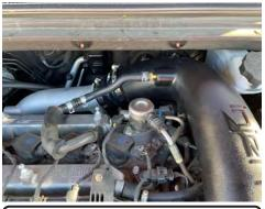
**18.** Reinstall the factory vacuum line onto the fitting located on the Injen intake tube
