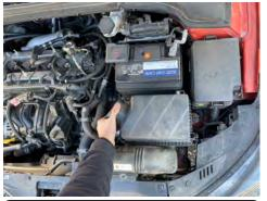
**8.** Remove the stock air box and scoop assembly from the engine bay
