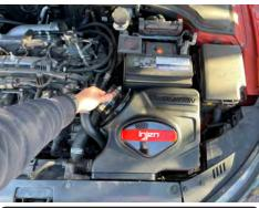
**14.** Place the Injen twist lock filter into the Injen air box. Make sure you rotate the filter until you feel it engage
