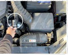
**2.** Detach the diverter valve return line from the stock intake tube
