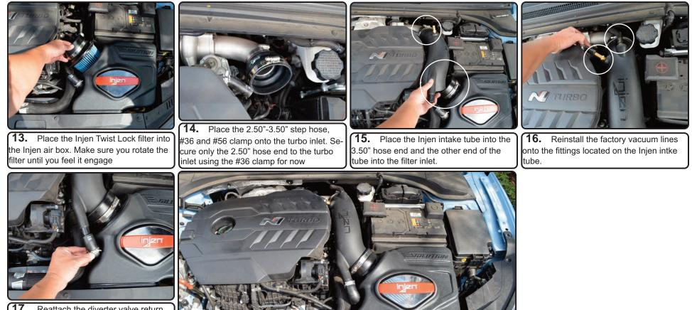
**17.** Reattach the diverter valve return line to the Injen Intake tube diverter valve port.
