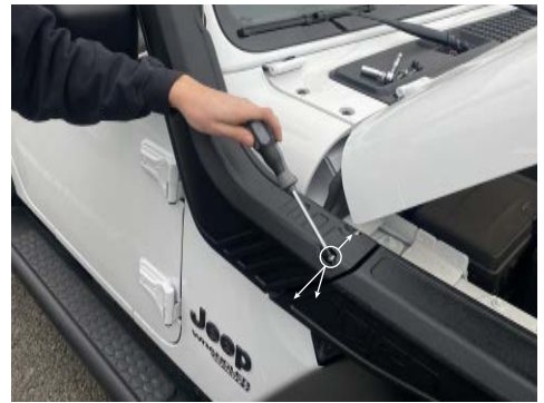
15. Secure the upper snorkel to the lower snorkel using four M6 phillips bolts
