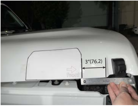
25. Tape the cutting template 3"(76.2mm) from the outer tangent point on the hood latch indentation. Then trace the template.
