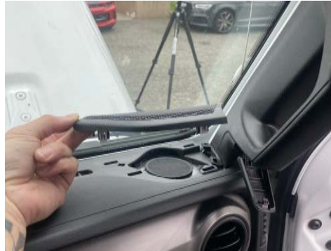
17. Unclip the speaker cover.
