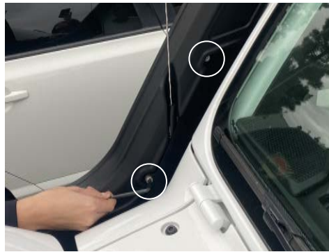
14. Bolt down the upper snorkel to the lower bracket using the provided M8 x 1.25 12mm bolts.
