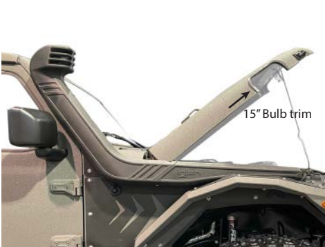
28. Place the bulb trim onto the edge of the cutout. Trim the bulb trim as needed.
