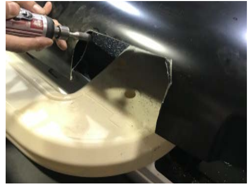
27. With a flat grinder clean up the edges and open up as needed for clearance.
