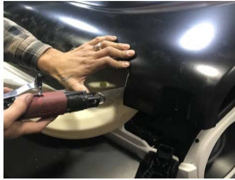
26. Use the traced line to cut the hood. Under cut the opening and repeatedly check clearance with the snorkel.
