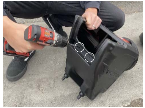
3. Drill out the two indents located on the back of the air box with a 9/32" drill bit.
