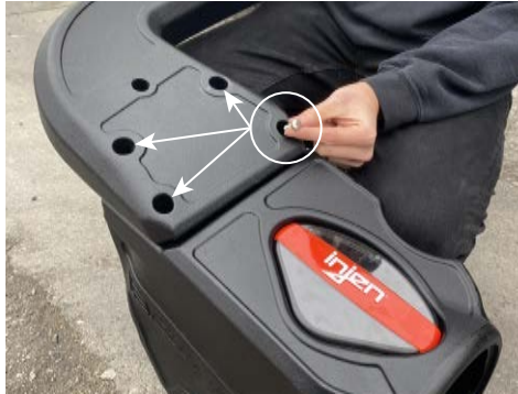
5. Bolt down the top of the lower snorkel using the provided four M6 phillips bolts.
