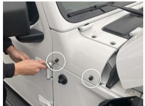
9. Remove the two OEM M8 torx bolts holding down the cowl panel.
