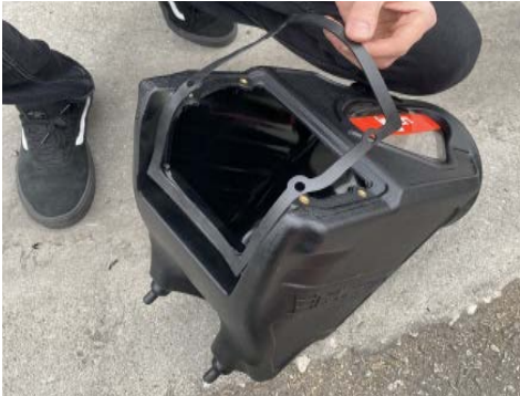
4. (OPTIONAL) Clean the gasket mating surface on the air box with rubbing alcohol then attach the gasket to the air box. Refer to advisory on pg. 2
