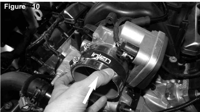
With clamps provided, attach the hose to the throttle body.
