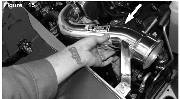
Figure 15 Install the intake assembly into the vehicle and position the bracket to the vibra mount and the throttle body.
