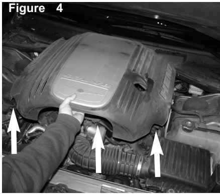
Lift up and remove engine cover.
