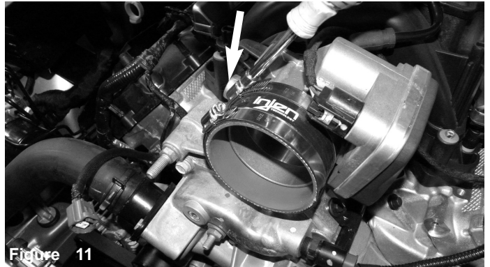
Use a 10mm socket with a 3/8 ratchet and remove the 10mm bolt mounting the factory air box to the radiator support.
