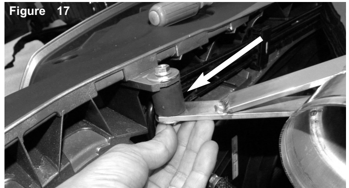
Figure 17 Secure the bracket to the bottom of the vibra mount using provided M6 nut and washer.
