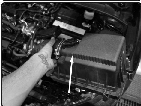
4. Now un-clip the upper part of the air box assembly. Lift up and remove from the vehicle.
