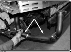
**25.** Carefuly remove the hot side intercooler pipe out of vehicle.
