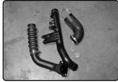
**11.** Complete cold side of intercooler pipe removed.
