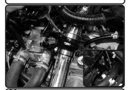
**20.** Adjust for the best fit, and tighten all clamps using 8mm nut driver.
