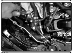
**23.** On back side of hot side intercooler pipe, locate the bolt holding in the intercooler pipe to bracket. Loosen and remove using 10mm socket and ratchet.
