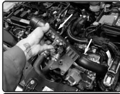
**7.** Carefully lift up and remove the upper intercooler pipe.
