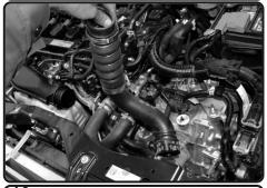
**10.** Remove the lower intercooler pipe out of vehicle.
