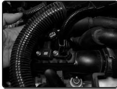
**3.** Disconnect both sensors on the upper intercooler tube.
