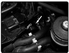
**12.** Install the 2.5" hump hose with clamps to the throttle body. Tighten the clamp on the throttle body only.
