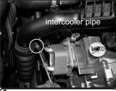
**6.** Loosen the clamp on the intercooler pipe using flat head screwdriver.
