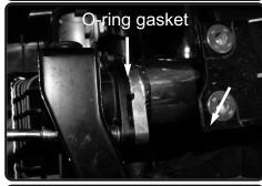
19. REMOVE FACTORY O-Ring gasket from OEM intercooler pipe and install to the new injen intercooler pipe. Connect the intercooler pipe flange to the intercooler using OEM bolts from step 9.
