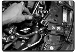
**22.** Loosen the clamp on the turbo using 10mm socket or wrench. Pull back the hose from turbo.
