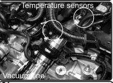
**21.** Re-connect the Temperature harness on engine. Re-connect both temperature sensor harness. Re-connect the vacuum line to the fitting on the intake tube and secure.
