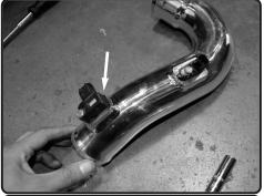
**15.** Install the 2nd temperature sensor into the last machined pad. Secure using provided M5 screw.
