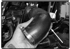
**8.** Now remove the 90 degree elbow hose out of the vehicle.
