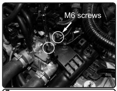
**7.** Use a 10mm socket or wrench and loosen the 2 bolts securing the upper intercooler pipe to the thermostat housing .
