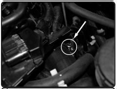
**4.** On OEM elbow hose, loosen the clamps on the throttle body using flat head screwdriver.
