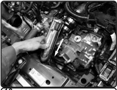
**18.** Install the lower intake assembly into the vehicle.
