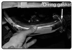
**28.** Install the injen intercooler pipe into vehicle.
