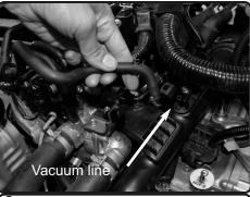
**2.** With pliers pull back the vacuum line from cold side of intercooler pipe.
