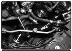
**30.** Attach the intercooler pipe from figure 28 to the elbow hose from figure 27. Once connected, secure with a clamp.
