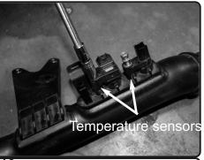
**13.** Loosen and remove the 2 M5 bolts holding in the 2 temperature sensors.
