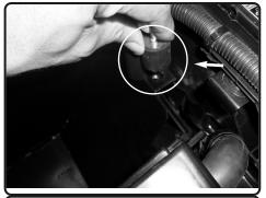
**30.** Now secure the back of the heat shield using M6 vibrmount.
