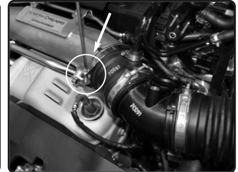
8. Loosen the clamp on turbo using phillips screwdriver.
