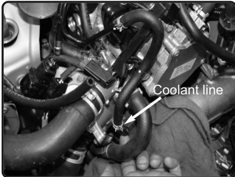
**17.** At other end of coolant line, Use a shop towel or rag, with pliers, loosen the clamp on the bottom of the coolant line. Pull Clamp backwards to be re-used.
