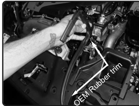
**26.** Remove the OEM rubber trim from the scoop using pliers. carefully pull out the clips holding in the rubber trim.
