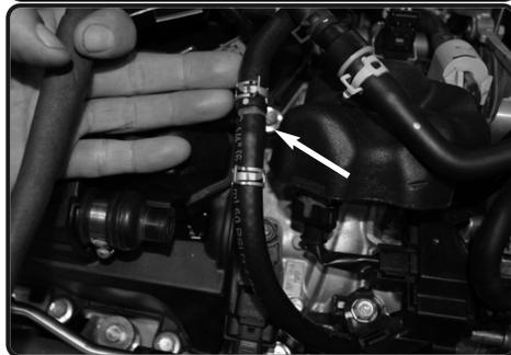
**23.** Connect the coolant line to the coupler from steps 15 & 16.
