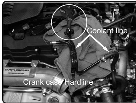
**14.** Use a shop towel or rag, with pliers, loosen the clamp on the top of the coolant line. Pull Clamp backwards to be re-used.
