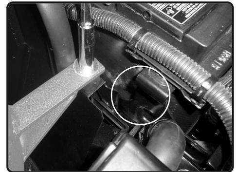
**40.** Secure the bracket using provided M6 nut and fender washer.
