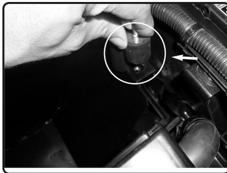
**30.** Now secure the back of the heat shield using M6 vibramount.
