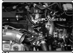
**24.** Verify and make sure the new coolant line is secured.
