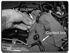
**15.** Pull back coolant line, now install provided 1/4" plastic coupler.
