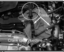
**14.** Use a shop towell or rag, with pliers, loosen the clamp on the top of the coolant line. Pull Clamp backwards to be re-used.
