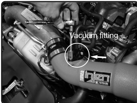
**42.** Secure the vacuum fitting using original screws from step 7.
