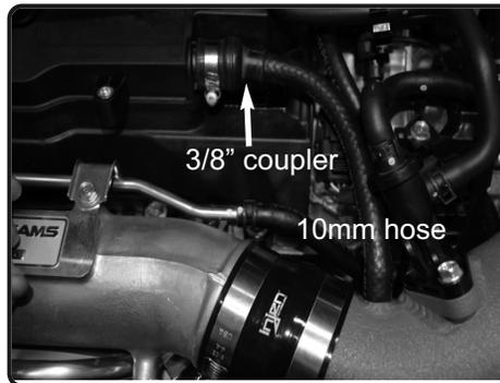
**43.** From step 13, connect the engine rubber coupler to the provided 10mm hose using provided 3/8" plastic coupler. Attach the 8mm hose to the fitting on intake tube. If hose is long, cut hose to correct 7" length. ***Make sure hose is not kinked or bend. May cause rough idle if hose is blocked or installed incorrectly.***
