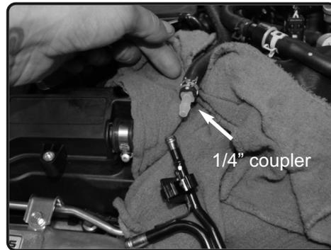
**16.** Install and secure the coupler using the OEM clamp from step 14.
