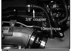
**43.** From step 13, connect the engine rubber coupler to the provided 10mm hose using provided 3/8" plastic coupler. Attach the 8mm hose to the fitting on intake tube. If hose is long, cut hose to correct 7" length. *Make sure hose is not kinked or bend. May cause rough idle if hose is blocked or installed incorrectly.*
