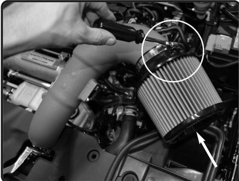
**37.** Install the air filter to the intake tube. Secure and tighten using 8mm nut driver.
