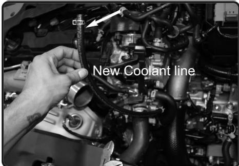
**21.** Remove another clamp from the OEM Hardline assembly, and install to the other end of the 6mm hose.
