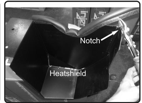
**28.** Install the rubber trim to the top of the heatshield, notch corner for easier installation.
