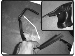
**27.** Complete OEM rubber trim removed. Remove the scoop.
