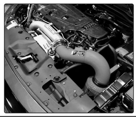
Congratulations! You have just completed the installation of this intake system. Periodically, check the alignment of the intake, normal wear and tear can cause nuts and bolts to come loose. <u>Note: Check clearance and adjust if needed! Failure to check the alignment and adjust the intake can cause damage that will void the warranty. Injen Technology is not responsible for any damages caused by/from improper installation.</u>
