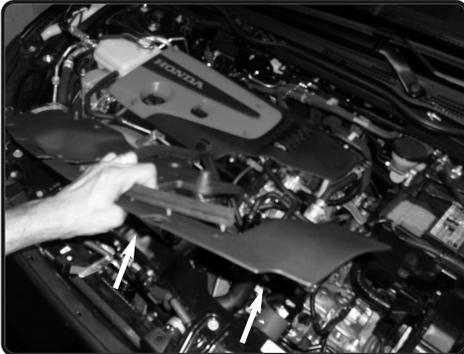
**25.** Remove the plastic push clips and remove the plastic radiator shroud.
