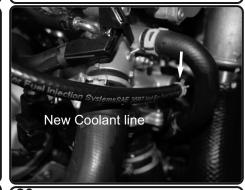
**20.** Install the clamp to the provided 6mm hose. Install and secure to the fitting from step17.
