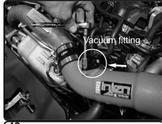
**42.** Secure the vacuum fitting using original screws from step 7.
