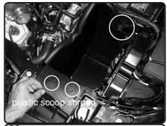
**29.** Install the heatshield and position. Make sure the heatshield sits on top radiator support. MAkes sure plastic scoop shroud sits on top of heatshield.
