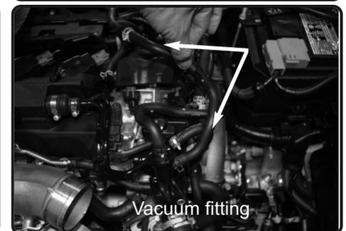
12. Now pull back vacuum line assembly out of way for the removal of the crankcase/coolant hardline.
