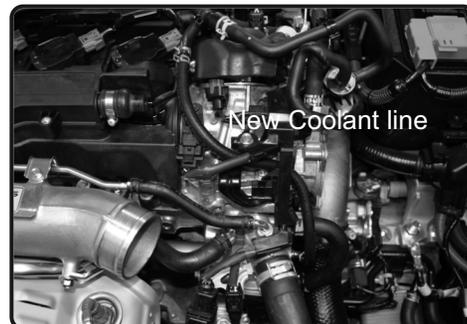
**24.** Verify and make sure the new coolant line is secured.
