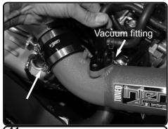
**41.** Atttach the vacuum fitting to the flange adaptor. Adjust intake tube and tighten the clamps using 8mm nut driver.
