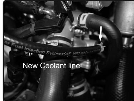
**20.** Install the clamp to the provided 6mm hose. Install and secure to the fitting from step 17.
