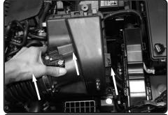
**10.** Lift up and remove the airbox.
