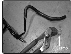
**19.** Remove clamp from the coolant line.
