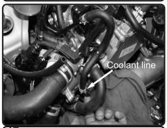
**17.** At other end of coolant line, Use a shop towell or rag, with pliers, loosen the clamp on the bottom of the coolant line. Pull Clamp backwards to be re-used.
