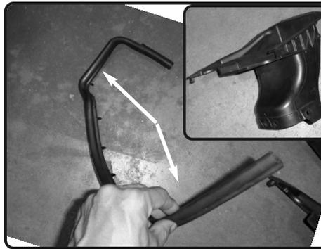
**27.** Complete OEM rubber trim removed. Remove the scoop.
