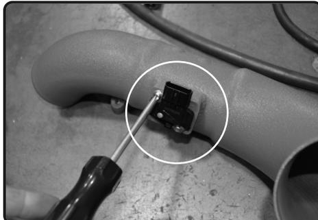
**34.** Install the MAF sensor into the new intake tube and secure using OEM screws. **Note: Make sure the sensor is going in the correct Direction!**
