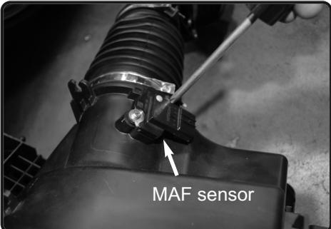
**33.** Loosen and remove the MAF sensor from the air box.
