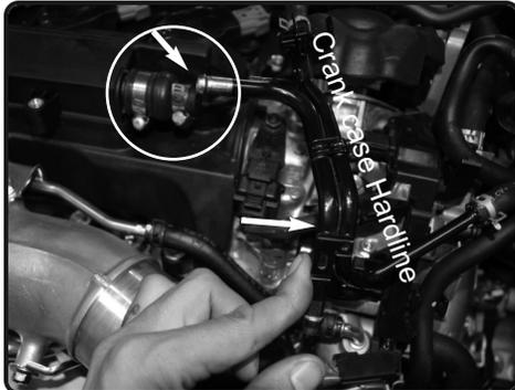
**13.** Brake the crank case clamp using pliers to remove. Pull the Crank case hard line out of the engine rubber coupler.
