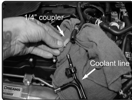
**15.** Pull back coolant line, now install provided 1/4" plastic coupler.
