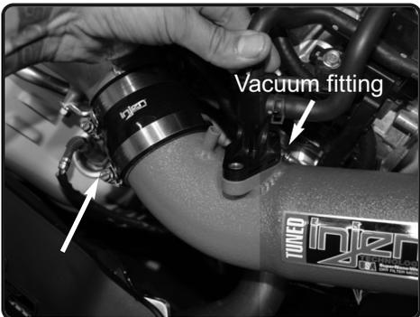
**41.** Attach the vacuum fitting to the flange adaptor. Adjust intake tube and tighten the clamps using 8mm nut driver.
