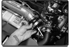
**35.** Install the provided step hose with clamps to the turbo.
