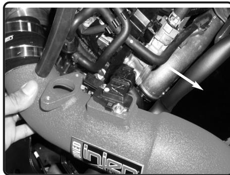
**38.** Install the intake assembly into the vehicle. Position the bracket to the vibramount and tube to the step hose.
