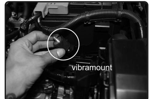
**36.** Install the provided M6 vibramount to the OEM airbox mounting bracket. Secure and tighten.
