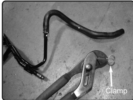
**19.** Remove clamp from the coolant line.
