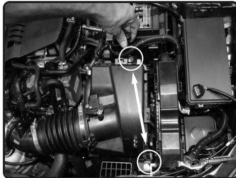
6. Loosen the two 10mm bolts holding in the stock air box.
