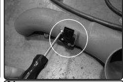
**34.** Install the MAF sensor into the new intake tube and secure using OEM screws. **Note: Make sure the sensor is going in the correct Direction!**
