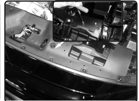
**32.** Secure and tighten screws using allen key. Re-install plastic radiator shroud.
