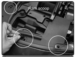
**3.** Carefully remove the push-clips from the upper engine cover.
