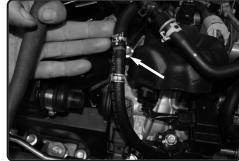
**23.** Connect the coolant line to the coupler from steps 15 & 16.
