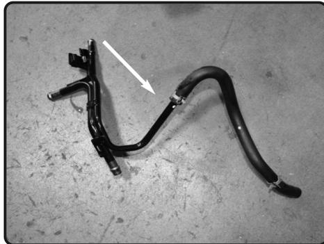
**18.** Remove the complete Crankcase/coolant hardline from fitting out of vehicle
