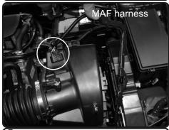
**5.** Disconnect the MAF sensor harness. Pull back the line away from the airbox.
