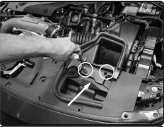
**2.** Loosen the 2 bolts holding in the OEM rubber Ram scoop.
