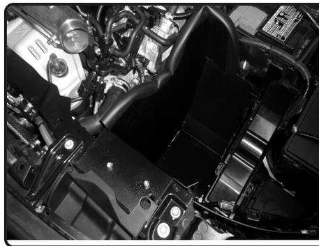
**31.** Secure the front of the heatshield using provided M6 socket cap screws.
