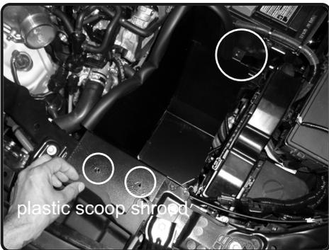
**29.** Install the heatshield and position. Make sure the heatshield sits on top radiator support. MAKES sure plastic scoop shroud sits on top of heatshield.
