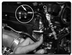
**13.** Brake the crank case clamp using pliers to remove. Pull the Crank case hard line out of the engine rubber coupler.
