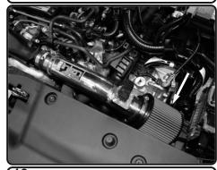
19. For extreme weather conditions, install filter on upper intake tube assembly for Short Ram Application.
