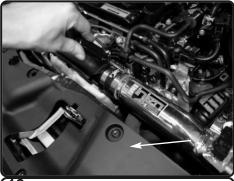
**18.** Tighten the clamp on straight hose.
