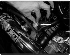
**15.** Secure the upper intake tube assembly bracket using M6 nut and fender washer.
