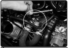
**9.** Locate the bracket on the engine holding in line. Pull back harness and loosen the bracket using 10mm socket or wrench.
