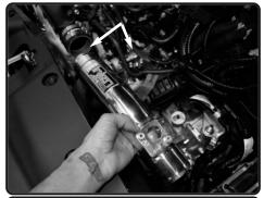
**14.** Install the upper intake tube assembly into vehicle and position tube to straight hose and bracket to vibramount.
